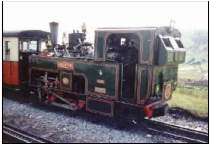
By re-draughting steam locomotives to our modern designs substantial benefits can be obtained! Savings of up to 30% in fuel and an increase of power up to 25%. Some locomotives have been re-draughted to reduce spark emissions and solve steaming problems with great success. We will install these types of chimney inside the existing chimneys so as to retain the traditional outline.
