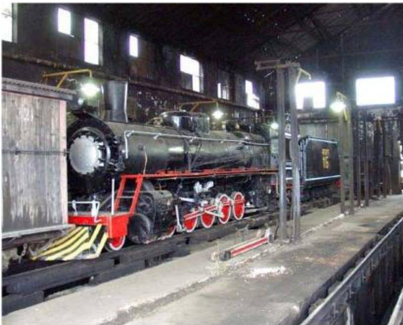
In 1963 a second batch of 2-10-2s were built for RFIRT by Mitsubishi. These machines incorporated all of Porta's modifications to the first batch plus some additional ones. On test these locomotives were able to show even better performance than the modified ones of the first batch.
